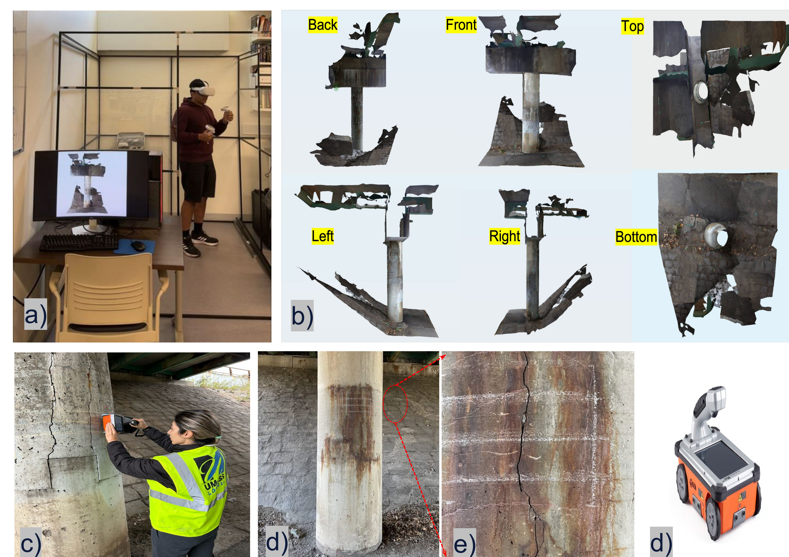
Fig. 1: a) VR chamber with a desktop computer; b) Point cloud data (PCD) models of bridge components; c) GPR field data collection; d) and e) The RC column (E3) for sample collection; e) GPR mini LT.
