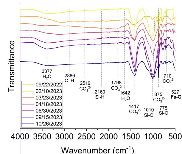
**Fig. 4:** FTIR results of samples collected from E3 column (sample collection location 1).
