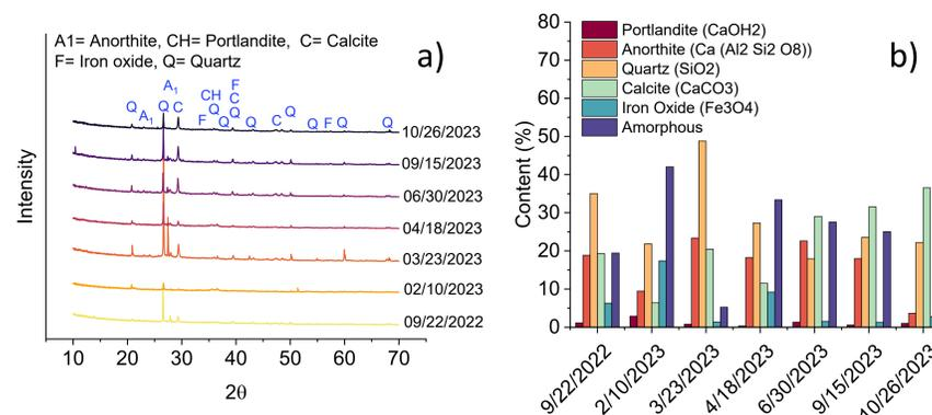
**Fig. 2:** XRD results of samples collected from E3 column (sample collection location 1).
