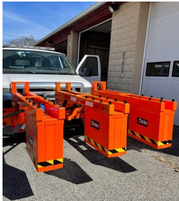
Figure 1: RIDOT Survey Van With and 3, 2GHz Antennas
