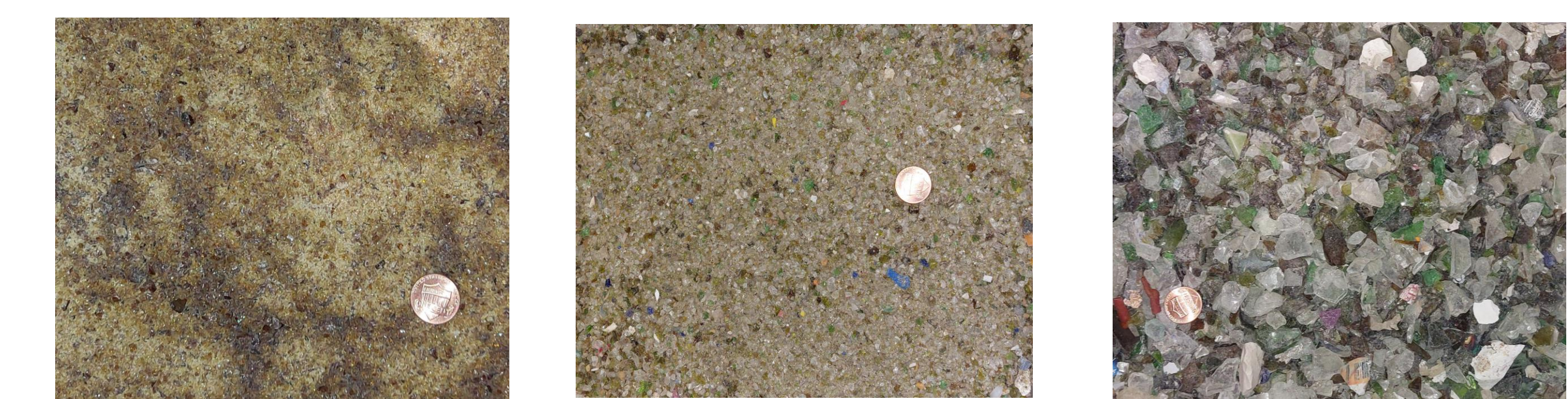
Figure 1: Lab manufactured PGA (Left), CSWD (Mid), New Hampshire PGA (Right) (A penny is included in photographs to provide a sense for particle size)
