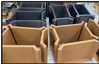
Figure 1: 3D Printed Formwork Sets
