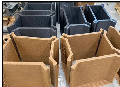
Figure 1: CF-ABS and WF-aPLA 3D Printed Forms
