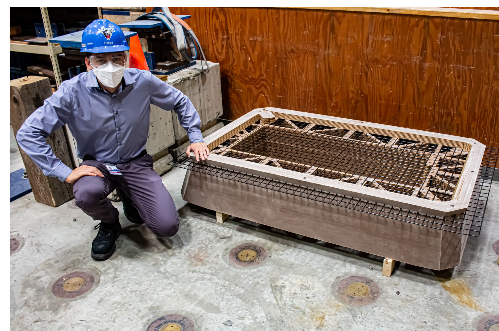
Figure 2: 3D Printed Formwork for Precast Concrete using WF/PLA material
