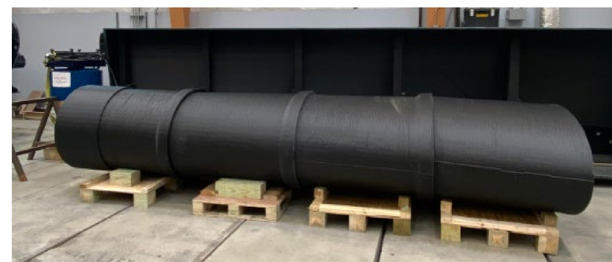
Figure 3: 3D Printed highway culvert diffuser using CF/ABS material
