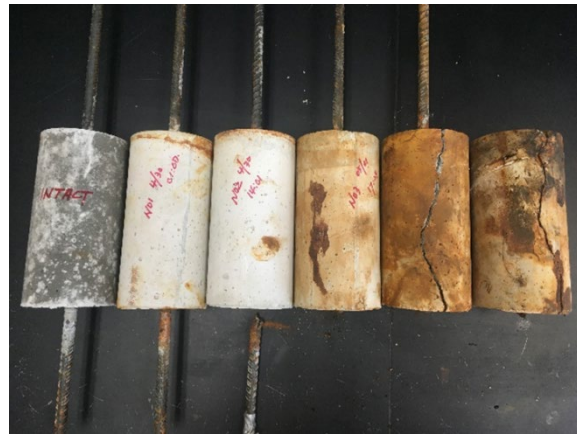
Figure 1: Comparison of Bond-Slip response of corroded and intact specimens (Left) and variations of corrosion degree produced by the accelerated corrosion test (Right).
