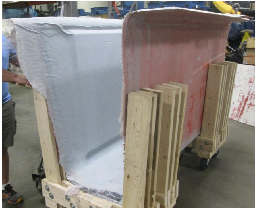
Figure 6: Infused, Cured Second Girder Mock-Up
