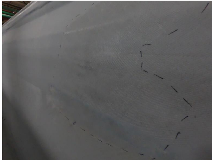
Figure 17: Debulked Structural Defect
