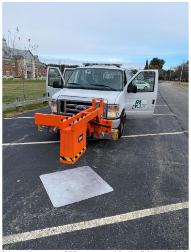
Figure 1. Calibration of the single-antenna GPR system used for the field work during the reporting period.
