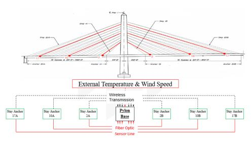
Figure 1: Data acquisition layout for carbon fiber composite strands in the Penobscot-Narrows Bridge
