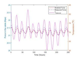
Figure 2: Predictive model of cable forces and temperature
