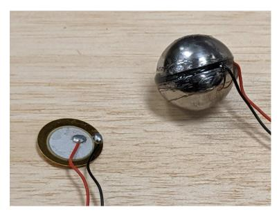
Figure 2 Piezoelectric sensor ball and embedded sensor disk
