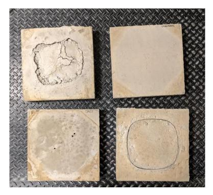
Figure 4. Concrete slabs with various forms of cast in place damage for laboratory testing.
