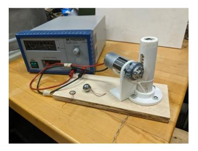
Figure 1. Rack and sector gear pinion steel ball tapper mechanism
