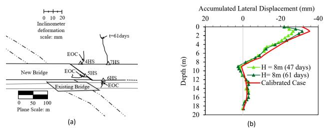
Figure 1. Lateral deformation in the CBIS field case: (a) plan view of inclinometer and its lateral deformation; (b) comparison of calibrated FEA model with measured displacements at location 7.
