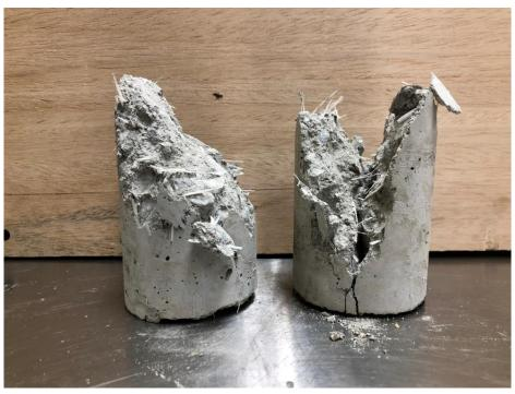
Figure 3 Concrete cylinder with fiber reinforcement following fracture testing
