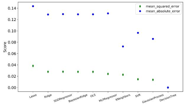
Figure 1 Comparison of different machine learning techniques in acoustic emission location performance in concrete
