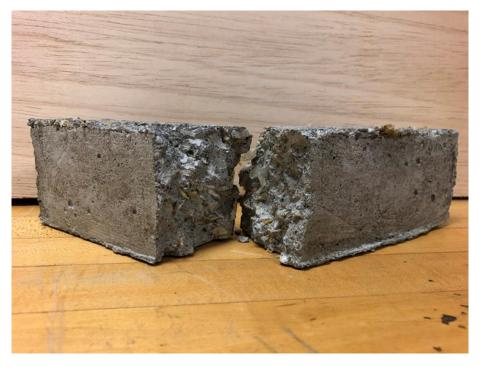
Figure 2 Concrete block sample following fracture testing
