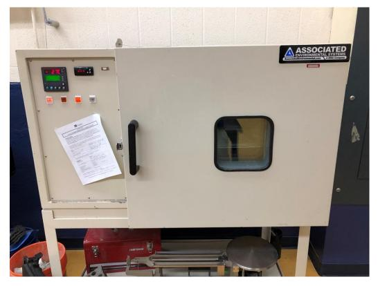
Figure 4 Environmental test chamber for freeze thaw testing of concrete samples
