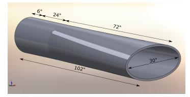
Figure 1: 3D model of the culvert diffuser prototype
