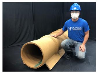
Figure 2: Ph.D. Candidate Sunil Bhandari with assembled 3D printed culvert diffuser
