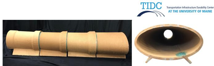
Figure 4: Side view and end view of assembled 3D printed culvert diffuser
