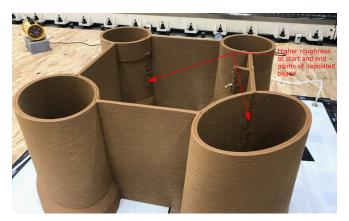
Figure 3: 3D printed culvert segment.
