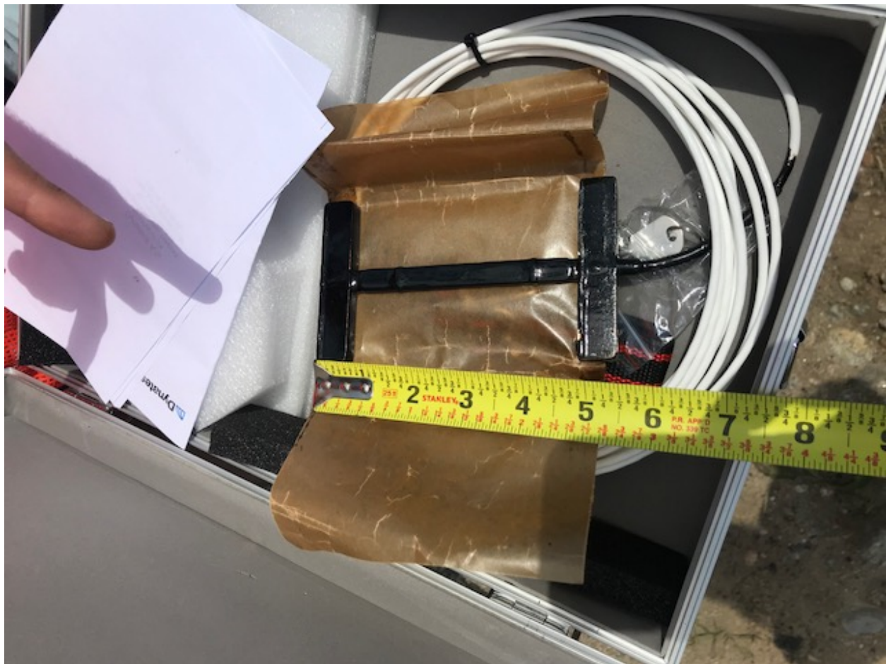
Figure 3.2. Dynatest Wheatstone bridge connection sensor
