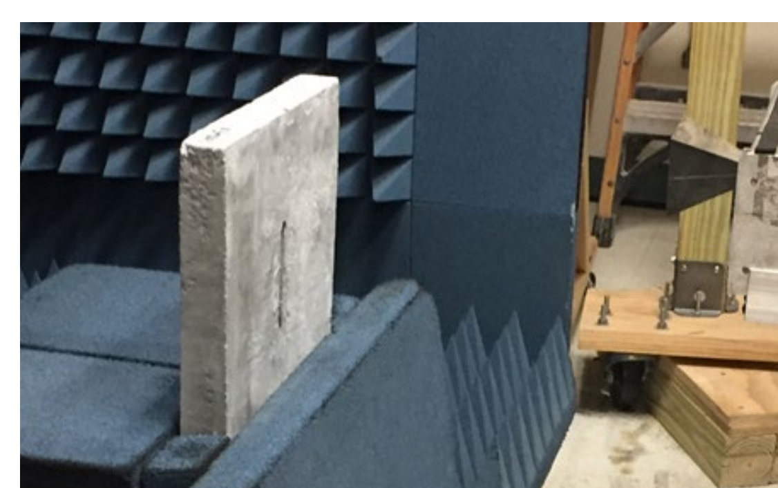
Fig. 2 Laboratory SAR imaging facility and SAR images of concrete specimens
