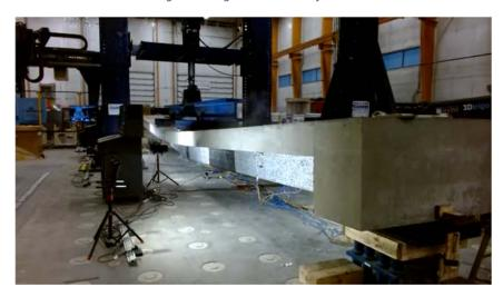
Figure 2: CT girder post failure
