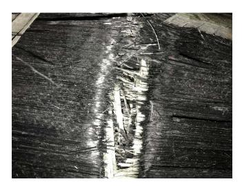
Figure 3: Close up of tension failure of the bottom flange
