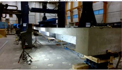
Figure 1: CT girder under test frame
