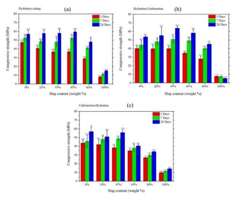
Figure 2: Cube compressive strength for different curing conditions (a) hydration, (b) hydration-carbonation, and (c) carbonation-hydration curing
