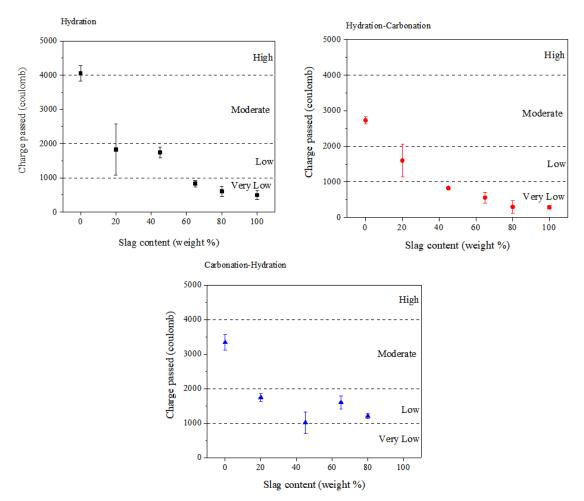
Figure 3: RCPT results of different curing conditions; (a) hydration curing, (b) hydration followed by carbonation, and (c) carbonation followed by hydration
