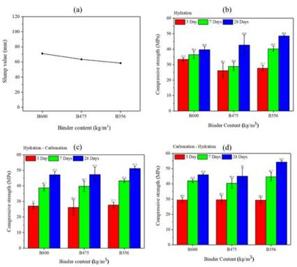
Figure 1: (a) Slump value with binder content, (b), (c), and (d) compressive strength of cylinders with different hydration, hydration-carbonation-hydration curing condition respectively
