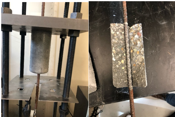
(a) Pull-Out UHPC specimens with un-corroded bar Figure 4. Pull-Out Test Results for Un-corroded bar
