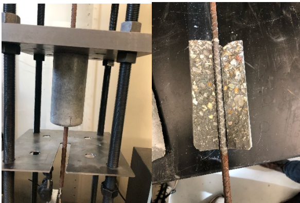
Figure 4: Pull-Out UHPC specimens with un-corroded bar.
