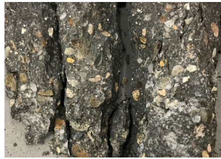
(a) Compressive strengths at 28 days (b) Failed surface of a specimen (c) Strength Development with Time Figure 1: Results of Compressive Strength Test
