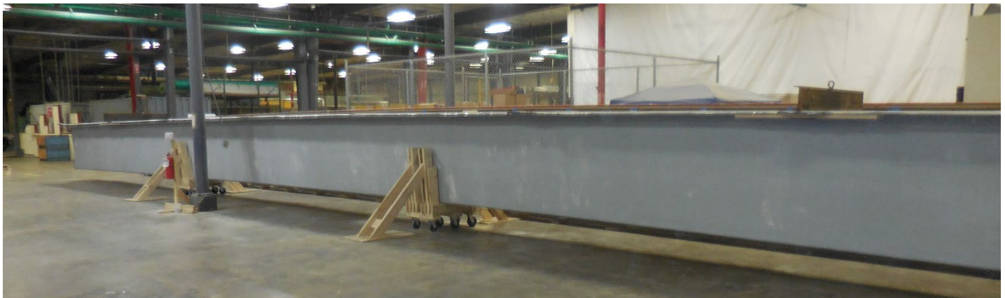
Fully infused and cured FRP tub-girder
