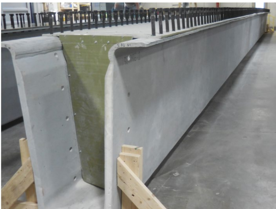
Fully infused, cured, and post-processed FRP tub-girder
