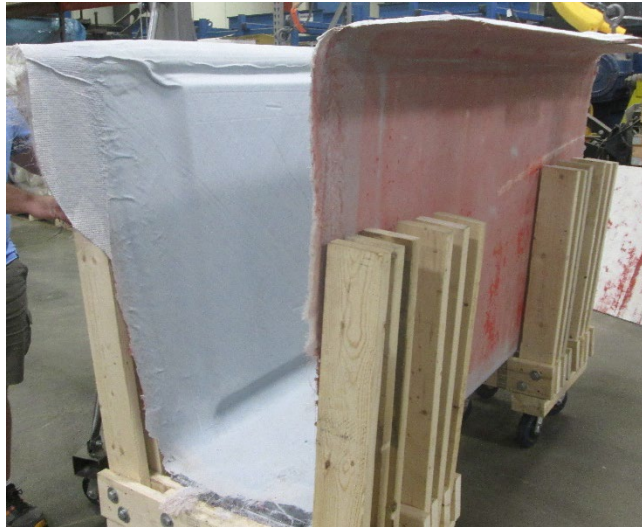
Figure 1: Completed Mock-Up Section of Girder
