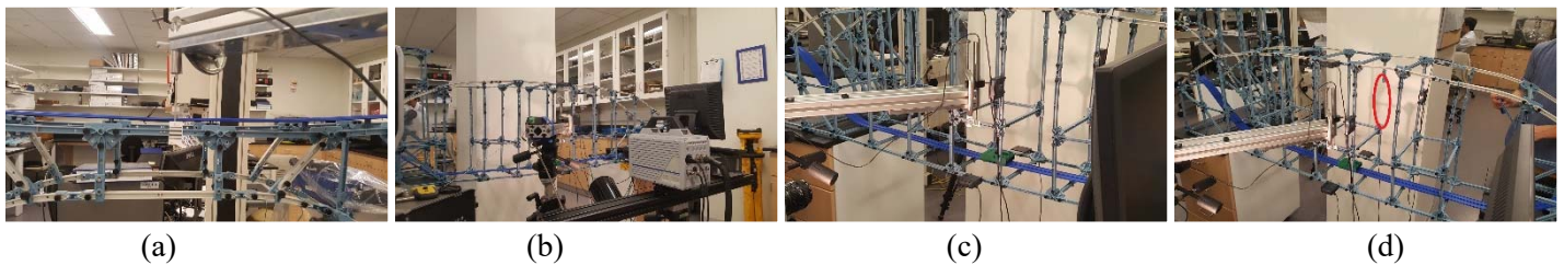
Figure 1. Bridge model testing with customized optical target. (a) and (b): two different bridge models with the setup of LVDT sensor and high speed camera; (c) and (d): zoom in of the optical target and damaged truss.
