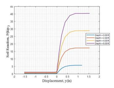
P-y Curves for the backfill of the sample IAB (GT STRUDL software)
