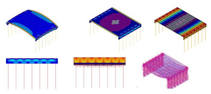
Contours for the sample single span IAB
