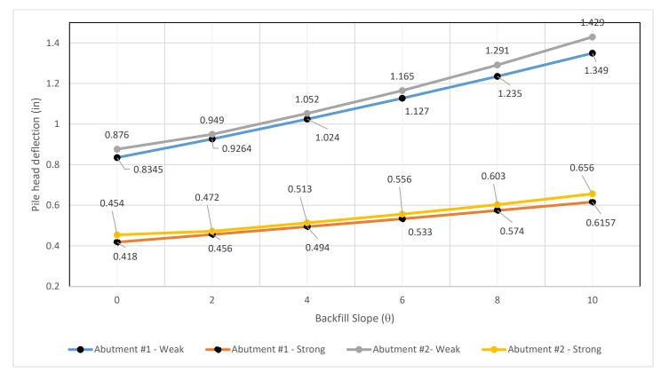
HP Piles head deflection vs range of slope (0-10%) for Bridge #38
