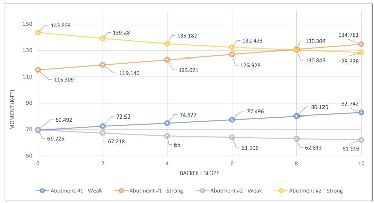
HP Piles head moment vs range of slope (0-10%) for Bridge #38
