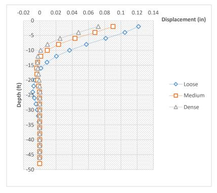
Deflection profiles for 50 ft. long HP pile for range of soil density
