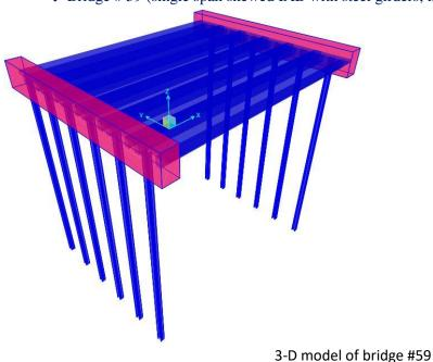
• Bridge # 59 (single span skewed IAB with steel girders, in the town of Dover, Vermont)
