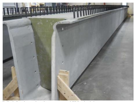
Fully infused, cured, and post-processed FRP tub-girder
