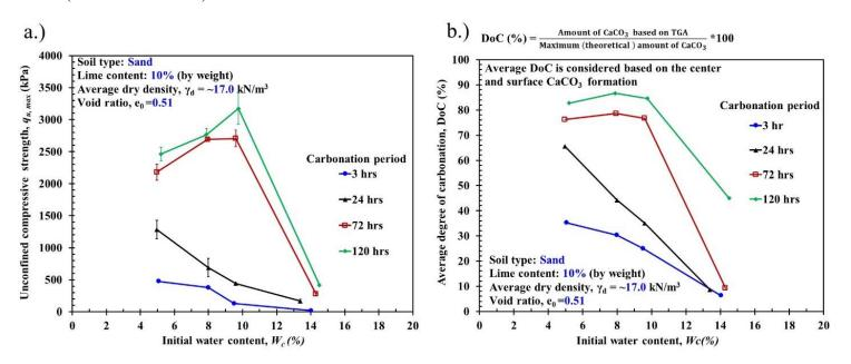
Figure 1. Effects of initial water content on a.) carbonated soil strength, and b.) degree of carbonation of 10% (by weight) lime-mixed sand specimens prepared at constant density/void ratio
