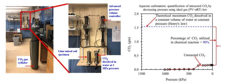
Figure 1. Laboratory test setup for aqueous based soil carbonation
