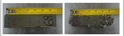
After 168 freeze-thaw cycles; 0.24 wt% active fiber specimen with minimal damage (left) and 2% passive fiber specimen with significant damage (right)
