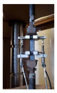
Fig:- Direct Tension Test Setup
