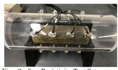
Fig:- Surface Resistivity Test Setup
