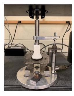
Fig:- Fiber Pullout Test Setup
