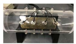
Fig:- Surface Resistivity Test Setup
