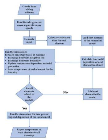
Figure 1. Flow chart of model developed to enable design of 3D printed parts
