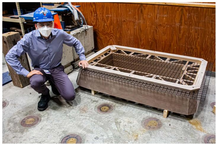
Figure 1. Felipe Saavedra, MS student in Civil Engineering with 3D printed form assembly
