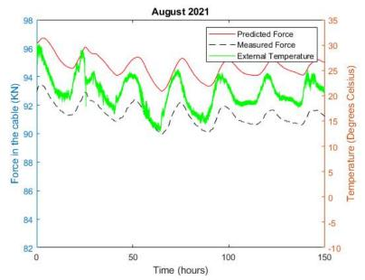
Figure 1. Force and temperature over time in a carbon fiber composite cable in stay 10B at the Penobscot Narrows Bridge
