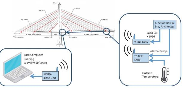
Figure 1. Wireless data acquisition schematic
