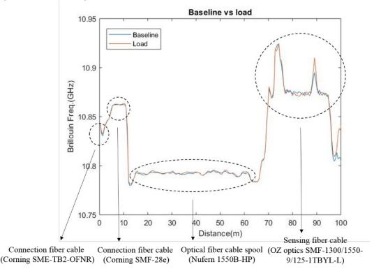
Figure 8. BOTDR results for the entire connected fiber cable area.
