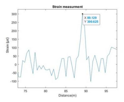
Figure 10. BOTDR results for the sensing fiber cable area in strain information.
