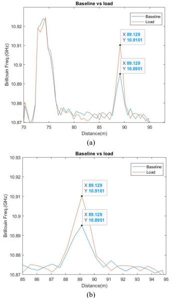
Figure 9. BOTDR results for the sensing fiber cable area.
