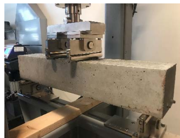
Fig. 1 b) Picture of 4- point bending
